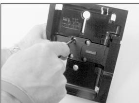
Using the HW4-R10 kit, attach the wiring bracket that came with the GPS to the inside of the Panel Dock. Tight securely but **do not over tighten the screws** - this may result in cracking of the bracket.
