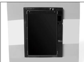
To install your GPS into the dock, gently snap it into place in the Mounting Bracket. After inserting, make sure the release lever is in the up position to keep the GPS in place.
